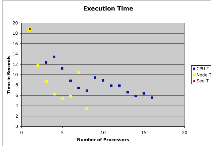
Figure 3 shows the performance evaluation on neuronic was run using 8 nodes. Two sets of performance data were collected. The NodeT set was collect using one processor per node and the CPUT set was collect using two processors per node.
